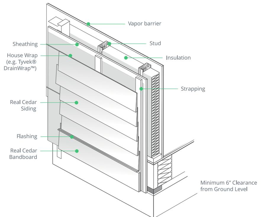
In all cases, high quality, corrosion resistant, ring or spiral shank siding nails **MUST** be used and they **MUST** be long enough so that they **PENETRATE SOLID WOOD** by a **MINIMUM** of 1 ¼”.
