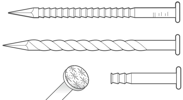
The size of nails to use depends on the type and thickness of siding. Use ring-shank siding nails long enough so that they penetrate solid wood by a minimum of 1¼”.
