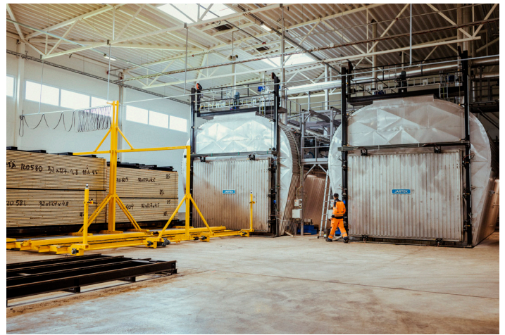
Thermal kilns at Loo production unit.
