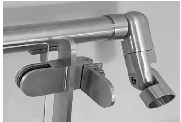
Transitioning from top rail to stair rail is accomplished with two pivots connected with a male joiner or short piece of rail pipe. Optionally, you may terminate the top rail with an end cap then install separate stair rail at the desired height.
