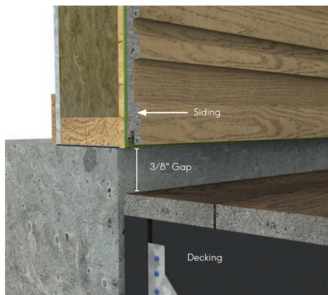
Fig. 7 - Install detail above deck
