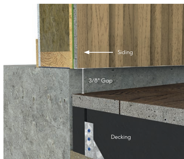
Fig. 7 - Install detail above deck
