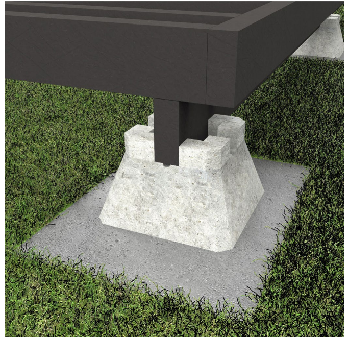
Fig. 15a - Pre-cast concrete pier
