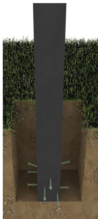
Fig. 12 - Plas-Pro frame screws in post
