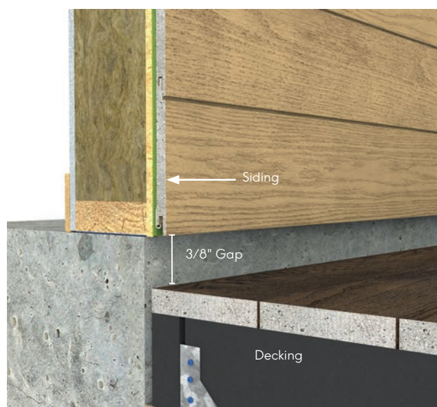
Fig. 7 - Install detail above deck
